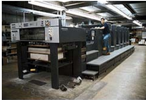
40" Heidelberg Speedmaster six-color press used by PrintTech, a division of York Graphic Services, Inc., for reproduction of P. Buckley Moss paintings. PrintTech uses the additional printing units to add varnish to Pat's four color posters.
