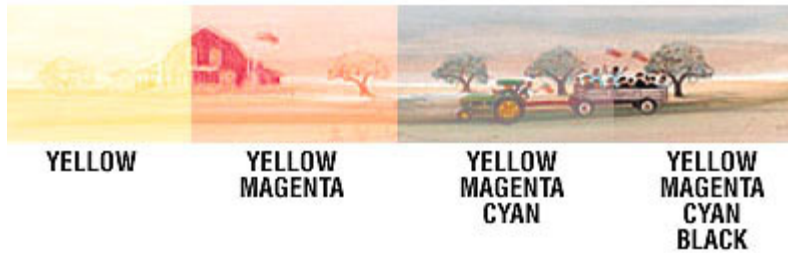
The Apple Barn has been printed in such a way to show how the four printing colors build upon each other to recreate a full color image.
